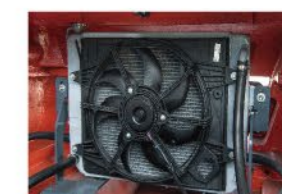
High efficiency liquid cooling and heat dissipation system is equipped as standard, which can meet the requirements of automobile S1 continuous working system;
