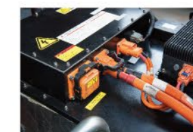
System level voltage safety protection: The truck features integrated / shortest design of voltage connection and multiple insulation monitoring protection; System level voltage safety sectional design: when the maintenance switch is pulled out, the system fails or the key is disconnected, the voltage system will be automatically disconnected, and the maximum voltage shall not be greater than 76.8V;
